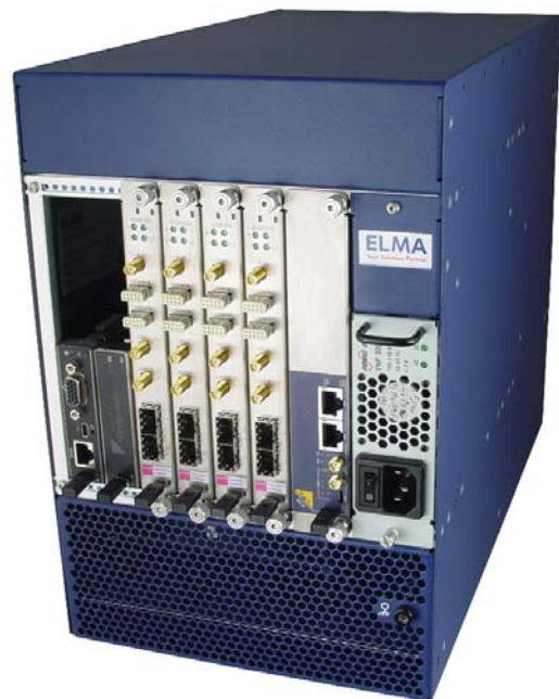
MTCA.4 ( \mu TCA for Physics) System with CPU, Disk, Digitizers and MCH
