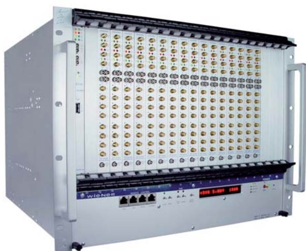
128 channel 1.25 GSPS 10-bit SIS3305 Digitizer system
