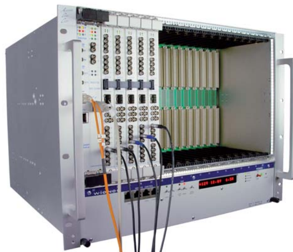
80 channel 250 MSPS 14-bit SIS3316 Digitizer system with front panel bus
