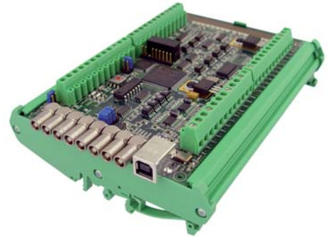
SIS9965 mounted in DIN rail fixture
