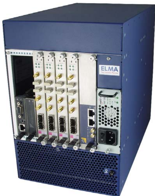
MTCA.4 ( \mu TCA for Physics) System with CPU, Disk, Digitizers and MCH
