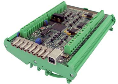
SIS9965 mounted in DIN rail fixture
